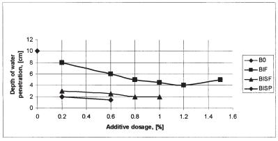
Fig. 6. Depth of water penetration under pressure (8 atm)
