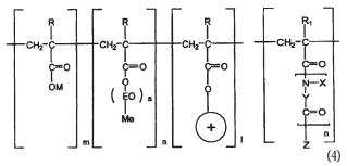
By changing the functional units in the chain, the effects of additives in concrete can be modified [6]. They are mainly used for the flow control and slump loss in the ready concrete as response to the users requests.
