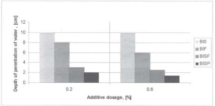
Fig. 7. Depth of water penetration under pressure (8 atm)
